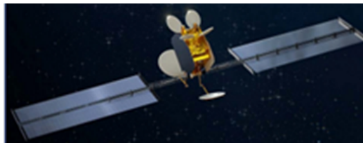
Figure 11.4: Deployable mast solar array [R.D. 3]
